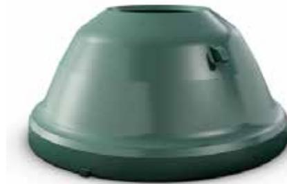
Example of normal wear. Obtained with correct feed arrangements, feed gradation and parameters for the cavity.
